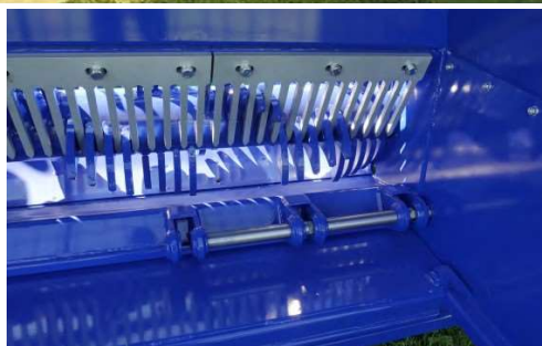
Hydraulic gudgeon pin for internal braking system with inside rope Replaceable rotor counter screens Hydraulic tunnel cleaning
