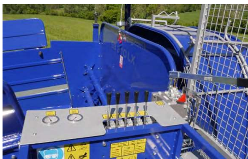
Synoptical control panel
